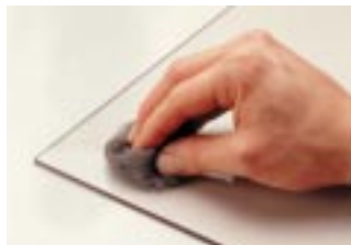
The wire wool test shows the superior performance of Lexan Margard sheet over conventional, uncoated sheet.
